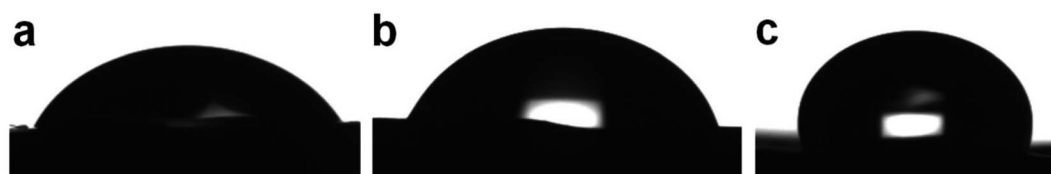
Fig. 9 Water contact angle measurements on the PU samples (a) PU-1, (b) PU-2 and (c) PU-3.
