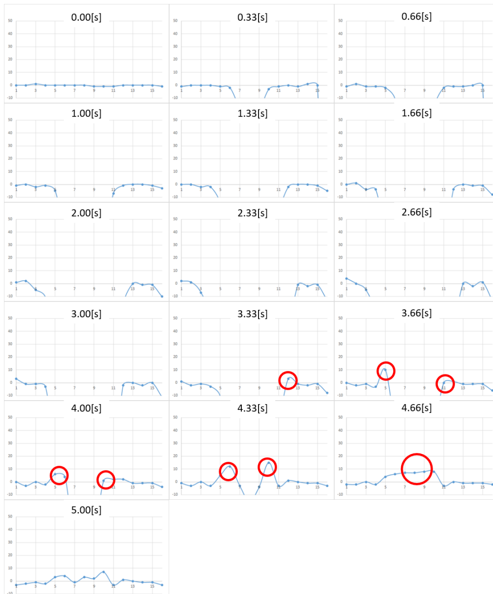
Figure 15. Change in pressure distribution for shampoo. The vertical axis represents the force (in milli newton). The horizontal plane represents the location of the sensing point.
