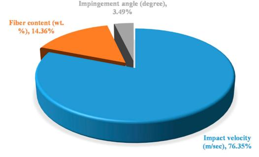
Figure 7. Contribution chart of factors for epoxy-based composites.
