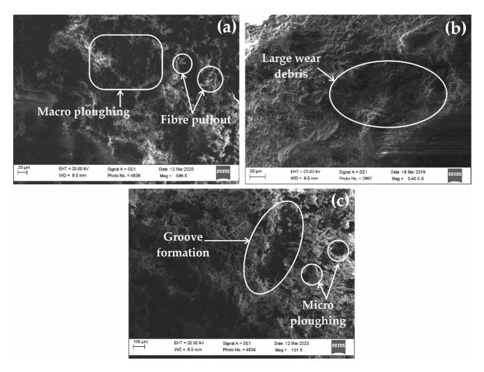
Figure 10. SEM images at highest fiber loading (a) epoxy based composite, (b) vinyl ester and (c) polyester based composite.
