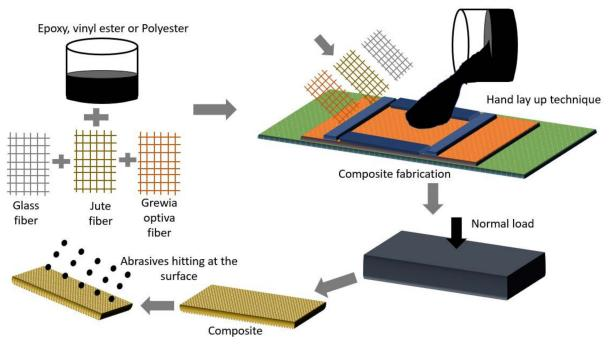
Figure 3. Process of fabrication of composite.
