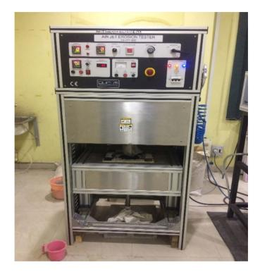
Figure 5. Air jet erosion test machine set up.
