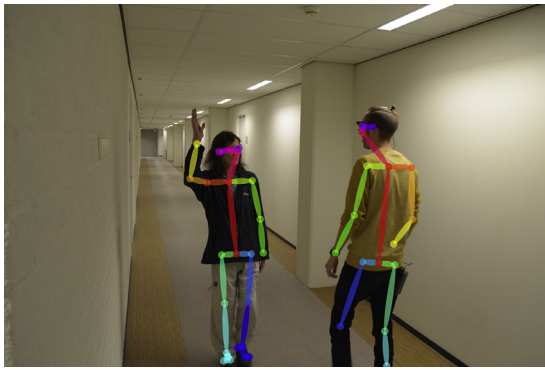
Figure 3. OpenPose body keypoints for one of the staged pictures of a walker-behavior. Note that not all keypoints are always identified (e.g., the missing left foot of the person in the yellow sweater). Note also that some keypoints are identified even if they are occluded (e.g., the right wrist of the person in the yellow sweater).
