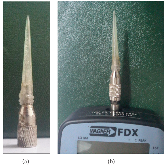
FIGURE 1: Tip made from 200 \mu\text{L} polypropylene micropipette tip filled with epoxy and mounted on a modified hook (a). The tip-mounted hook was screwed onto the algometer (b).
