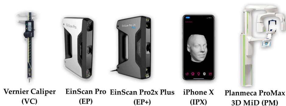
Figure 4. Vernier caliper and various face scanners used in this study. EinScan, EinScan Pro 2X Plus, iPhone X, and Planmeca ProMax 3D Mid.
