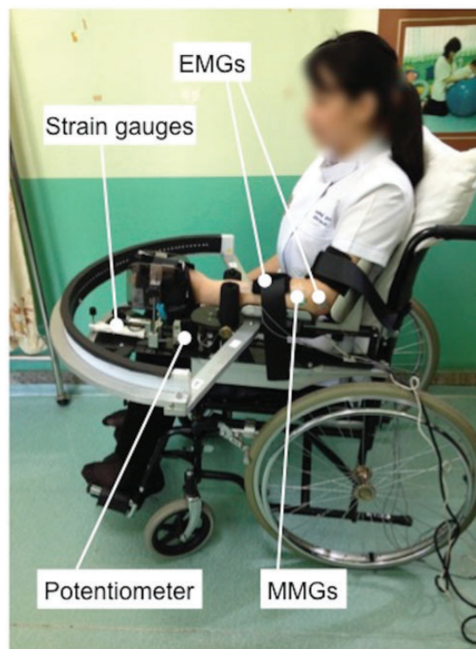
Figure 2. Participant set-up in the wrist rig showing force sensors, angle sensors, sEMG attached to the skin over forearm flexors and placement of MMG sensors over the forearm flexors. EMG: electromyography; MMG: mechanomyography.
