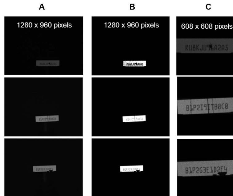
Figure 6. OCR data preparation. (A) original captured images with variations of image contrast and shifting of region of interest (ROI), (B) thresholding and edge detection, and (C) ROI cropping and padding.
