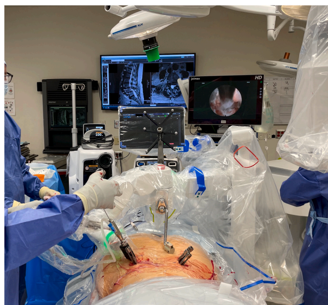
Fig. 1. This intraoperative photograph demonstrates the operating room setup with the Mazor Robot and endoscope monitor display at the foot of the bed. This allows for visualization of both the endoscope and navigation display in tandem. The optical camera for the Medtronic Stealth Navigation is placed above the anesthesia curtain, which is not shown in this picture.
