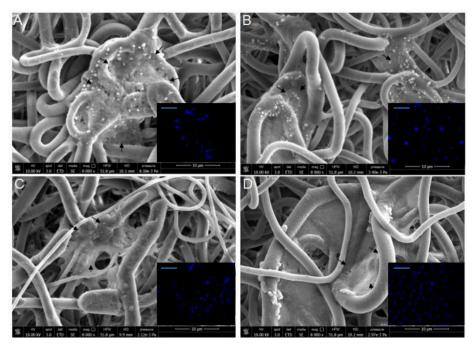
Figure 5. SEM and fluorescence (in inserts) analyses of P(VDF-TrFE)/HUVEC construct: (**A**) cell/scaffold construct (control); (**B**) cell/scaffold construct + OLE; (**C**) cell/scaffold construct +  $H_2O_2$ ; and (**D**) cell/scaffold construct + OLE +  $H_2O_2$ . Black arrows indicate the HUVECs in the construct. The scale bar in inserts is 100  $\mu$ m.
