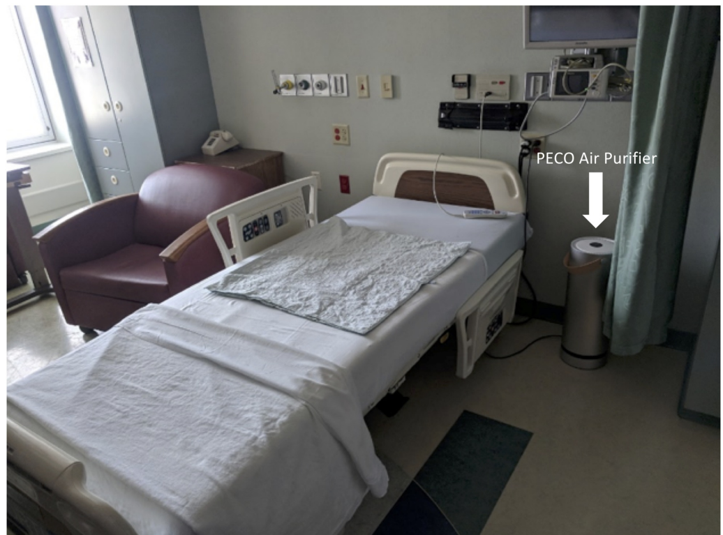
FIGURE 1: PECO portable air purifier placement in the patient room near the head of the bed
