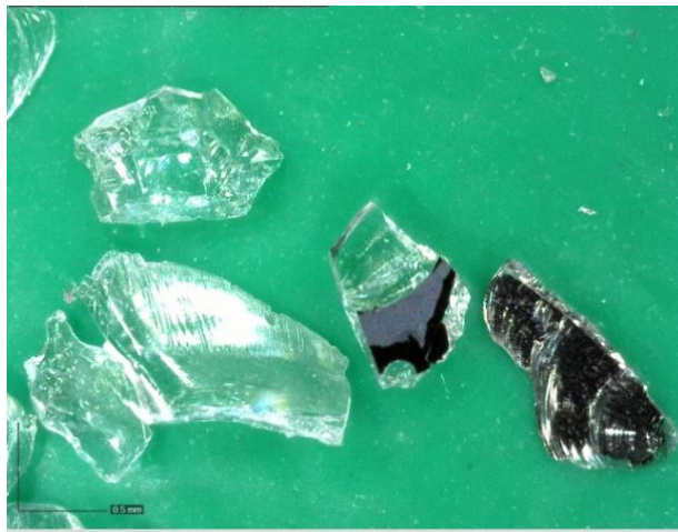
Figure 2. Glass recyclate fraction 0.5/1 mm; 103× magnified.
