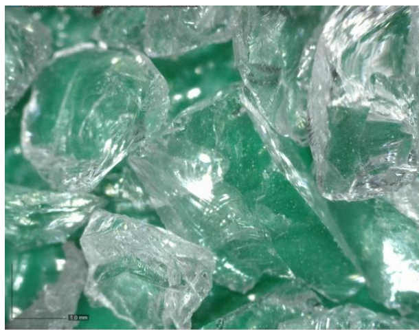
Figure 3. Glass recyclate fraction 1/4 mm; 51× magnified.
