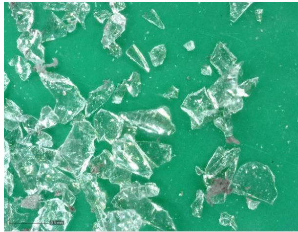
Figure 1. Glass recyclate fraction 0.0/0.5 mm; 103× magnified.
