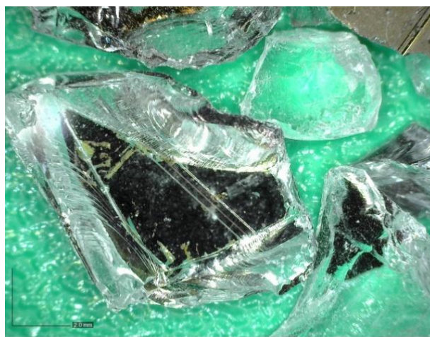
Figure 4. Glass recycle fraction 4/10 mm; 51× magnified.
