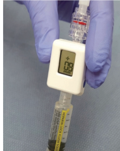
Fig. 1. Compact manometer used for endoscopic ultrasound-guided portal pressure measurement (Cook Medical, Bloomington, IN, USA).
