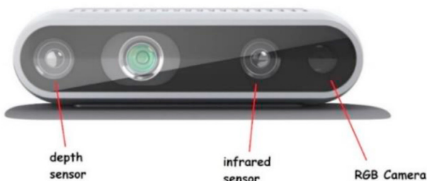
Figure 6. RGB-D camera named Intel Real Sense D430.
