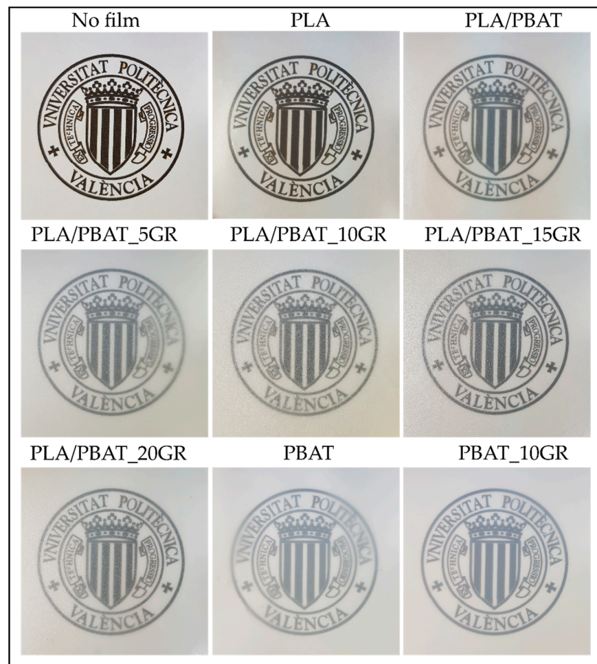
Figure 1. The visual appearance of PLA, PBAT, PBAT_10GR, PLA/PBAT, and PLA/PBAT with 5, 10, 15, and 20 phr GR resin films.
