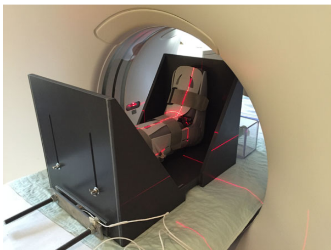
Figure 3. Controlled ankle motion boot inside the loading device.
