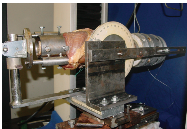
Figure 2 - Image of the knee fixed to the device.
