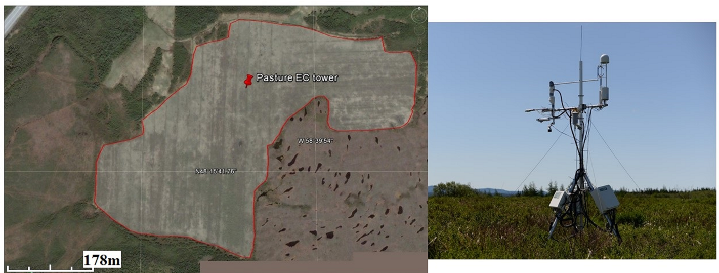
Fig 1. The location of flux tower in the Robinsons pasture, western Newfoundland, Canada (48.264 N, 58.665 W). The image is similar, but not identical, to the original image, and therefore is only for illustrative purposes. The outline of the site was indicated by the red solid line and the red pin represents the location of eddy covariance (EC) tower (a); (b) a photo of the setup of EC measurement system.
