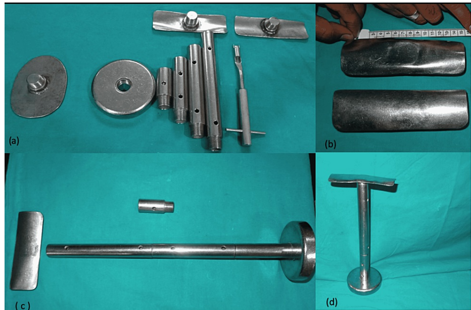
FIGURE 1: Components of modular tibia stand.
