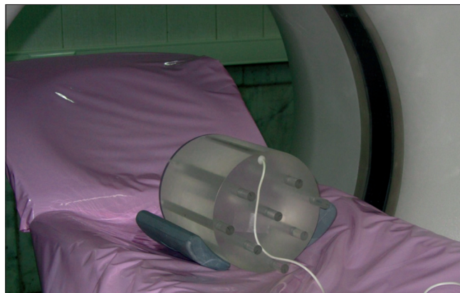
Figure 2: Computed tomography dose index phantom and an ion chamber placed in position of 12 o'clock
