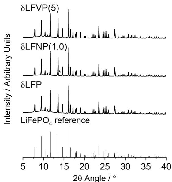
**Figure 2.** X-Ray diffraction patterns of  $\delta$ LFP,  $\delta$ LFP(1.0) and  $\delta$ LFP(5) with an  $\text{LiFePO}_4$  standard (PDF Card No. 01-070-6684), with the  $\text{Fe}_2\text{P}_2\text{O}_7$  minor impurity phase peak (PDF Card No. 00-076-1672, present in 1.5 vol% from Rietveld refinement) highlighted with an asterisk. A more detailed figure of the impurity phase peak is shown in Figure S2.
