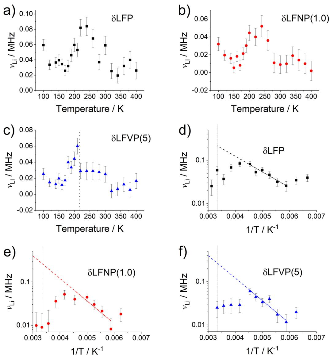
**Figure 4.** Plots of muon fluctuation rates  $\nu_{Li}$  vs Temperature for (a)  $\delta$ LFP, (b)  $\delta$ LFNP(1.0) and (c)  $\delta$ LFVP(5). Extrapolations of the muon fluctuation rate  $\nu_{Li}$  to room temperature on a log plot (indicated by the dotted line) vs inverse temperature ( $1/T$ ) for (d)  $\delta$ LFP, (e)  $\delta$ LFNP(1.0) and (f)  $\delta$ LFVP(5).
