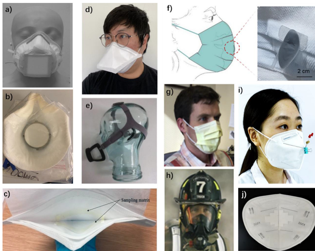
Fig. 4. Representative facemask devices for in vivo sampling of human exhaled breath aerosol: a) FFP3 facemask with a filter, reproduced from Ref. [28] with permission; b) FFP1 facemask with gelatin filter, reproduced from Ref. [32] with permission; c) surgical facemask with dog-bone specimen, reproduced from Ref. [33] with permission; d) Duckbill face mask fitted with PVA matrices, reproduced from Ref. [49] with permission; e) A filter held by a CPAP-type face mask, reproduced from Ref. [51] with permission; f) Wearable collector with facemask, reproduced from Ref. [53] with permission. g) Paper facemask, reproduced from Ref. [60] with permission; h) hard-surface plastic facemask, reproduced from Ref. [60] with permission; i) SPME fibers in KN95 facemask, reproduced from Ref. [46] with permission; j) paper strips in KN95 facemask, reproduced from Ref. [62] with permission.
