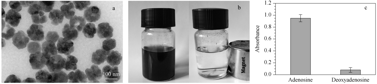
图 2 PEI-BA-MNPs 的 (a) 透射电子显微镜照片、(b) 磁分离照片和 (c) PEI-BA-MNPs 结合腺苷、脱氧腺苷的能力考察 ( n=3 ) Fig. 2 (a) TEM image and (b) photographs of magnetic separation of PEI-BA-MNPs and (c) investigation on the binding affinity of PEI-BA-MNPs to adenosine and deoxyadenosine ( n=3 )
