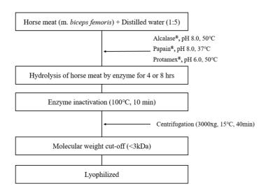
Fig. 1. Manufacturing procedure of horse meat hydrolysates.
