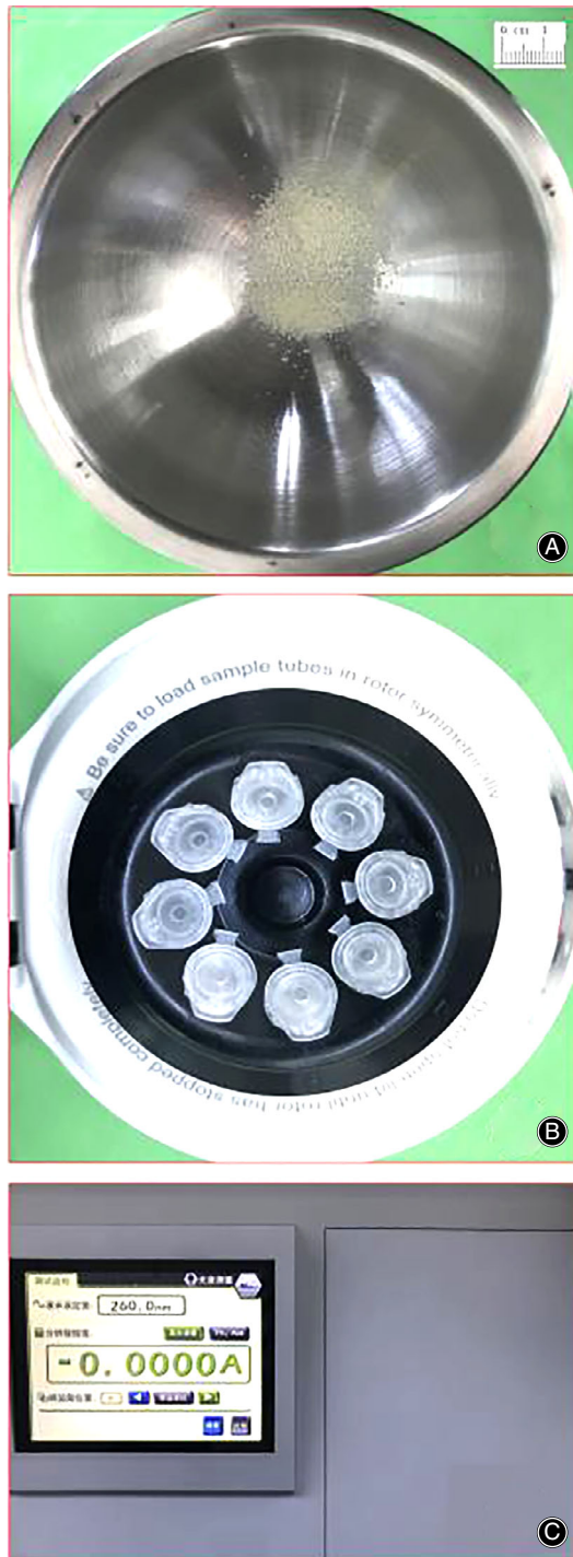
Fig. 1 DNA content determination process: grinding bone mass (A), centrifugation (B), and UV spectrophotometer to measure OD (optical density) value (C). Bone mass was ground to bone powder with a diameter of 0.80–1.50 mm. When centrifuging, we put the balanced centrifuge tube symmetrically into the centrifugal rotor (position balance), covered the centrifugal rotor, and paid attention to whether it was tight. The wavelength setting value of the ultraviolet spectrophotometer was 260.0 nm, and it was adjusted to “zero” after the setting was completed.
