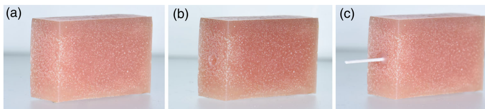
FIGURE 6 The block used in the pull-out test (a), a hole drilled in the center of the block (b), with the retainer wire bonded (c)
