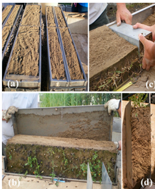
Figure 9. Growth boxes of Full (a, left) and Aerial (b, right) treatments; side front removal from a growth box at harvest (b); a soil column during (c) and after excavation (d).
