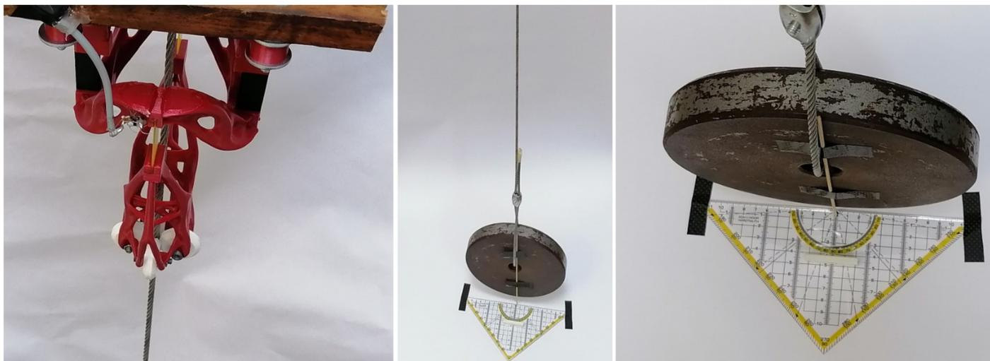
**Figure 4.** Measurement description: on the left, the sensing device; in the middle and on the right the detail on the ruler and pointer is shown.
