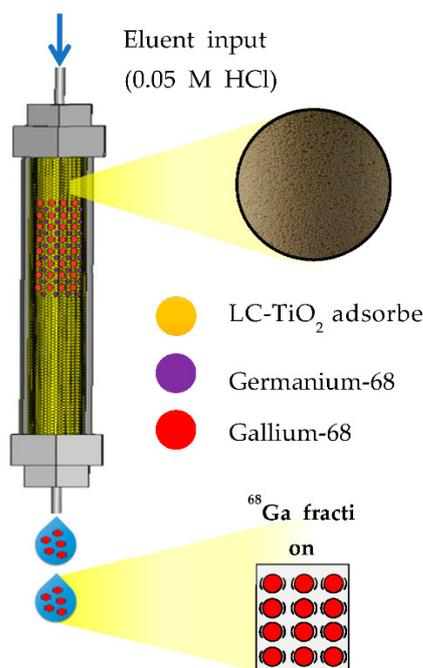
**Scheme 1.** Scheme of a  $^{68}\text{Ge}/^{68}\text{Ga}$  generator column system based on the chitosan- $\text{TiO}_2$  adsorbent.
