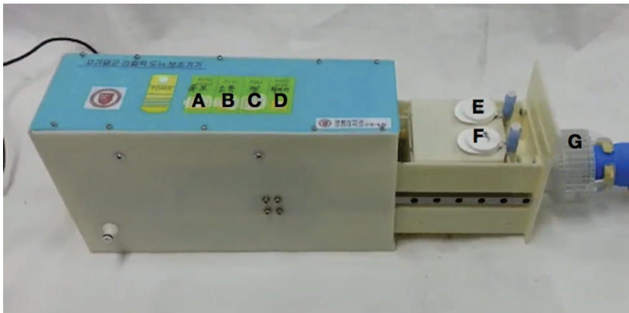
Figure 3. A prototype of the novel automatic urinary catheterization device. (A) Catheter progress and retraction button. (B) Sterilization button. (C) Lubrication button. (D) Start and finish button. (E) Chamber for lubricant. (F) Chamber for antiseptic agent. (G) Penis cap.
