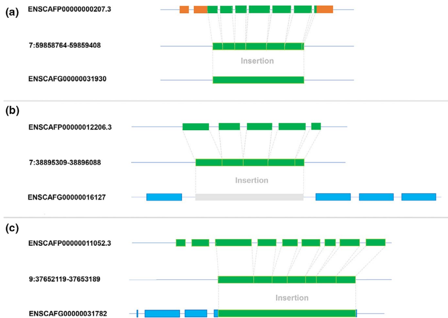
FIGURE 3 Three types of retrotransposition events. (a), (b), and (c) represent three types of retrotransposition events, respectively. Green boxes indicate coding sequence regions; orange boxes indicate UTR regions; blue boxes indicate new recruited coding sequence regions; gray box indicates a retrocopy inserted into the intron region of another gene
