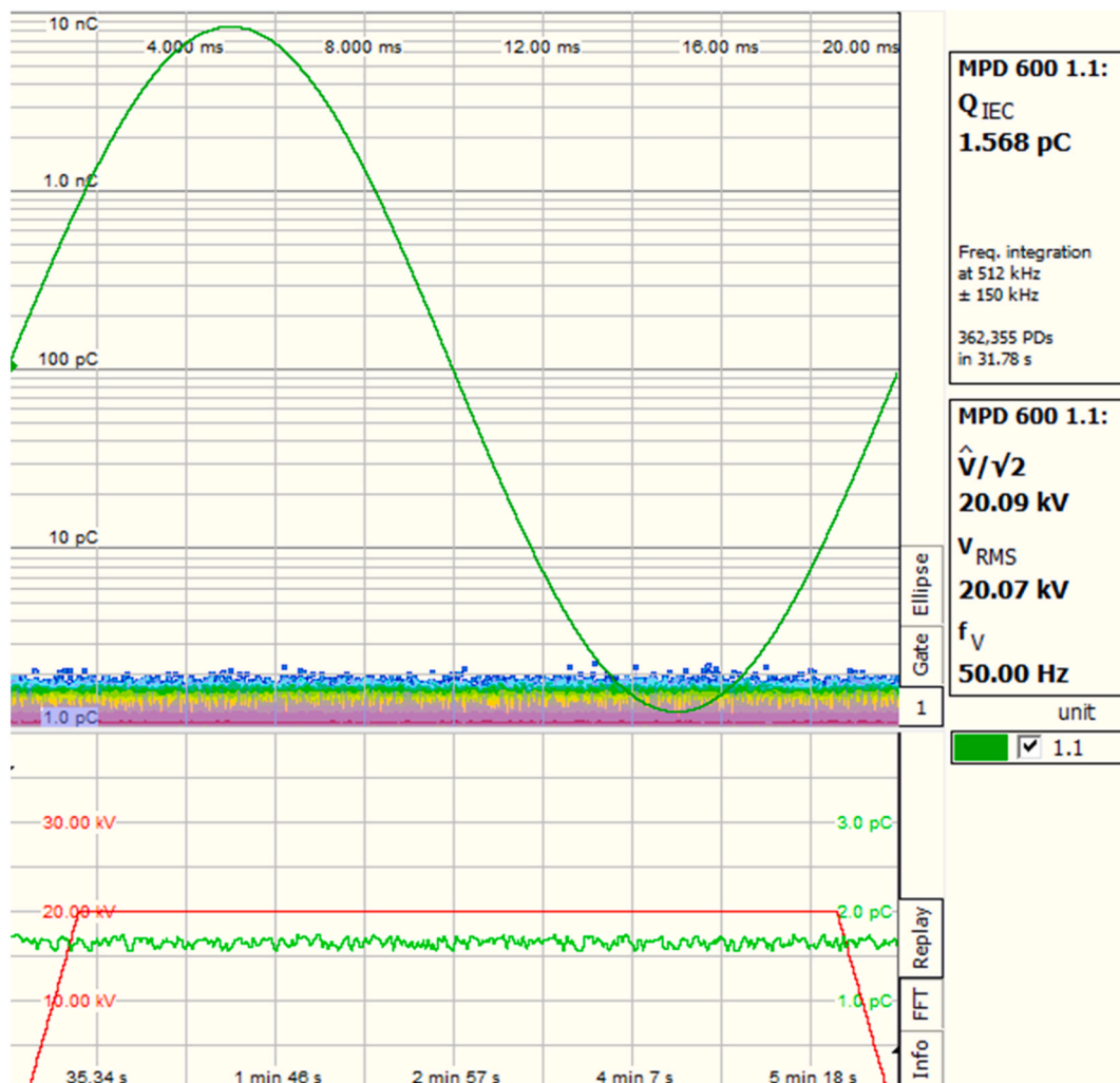
Fig. 4. Value, course of disturbance during measurement of partial discharges and behaviour of the voltage ramp.
