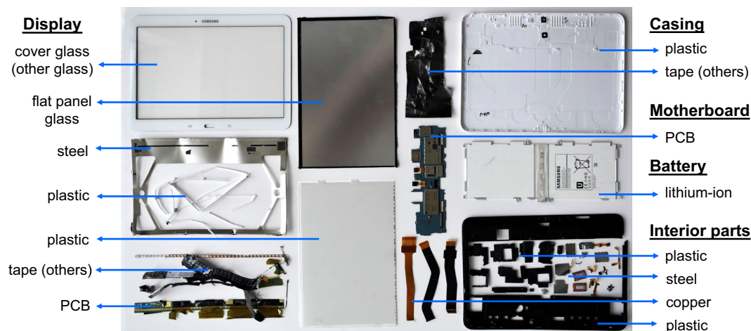
Fig. 1 Example of product disassembly for a tablet (Samsung Galaxy Tab 4 SM-T530, 2014), illustrating the disaggregation achieved via lab disassembly and physical identification and measurement of representative assemblies (underlined terms), components, and materials.
