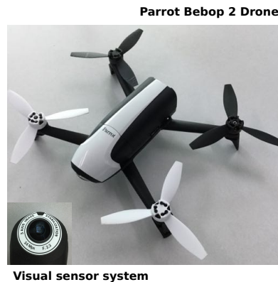
Figure 5. Parrot Bebop 2 Drone with a 14-Mpx flight camera. In the bottom-left corner, we show its visual sensor system.
