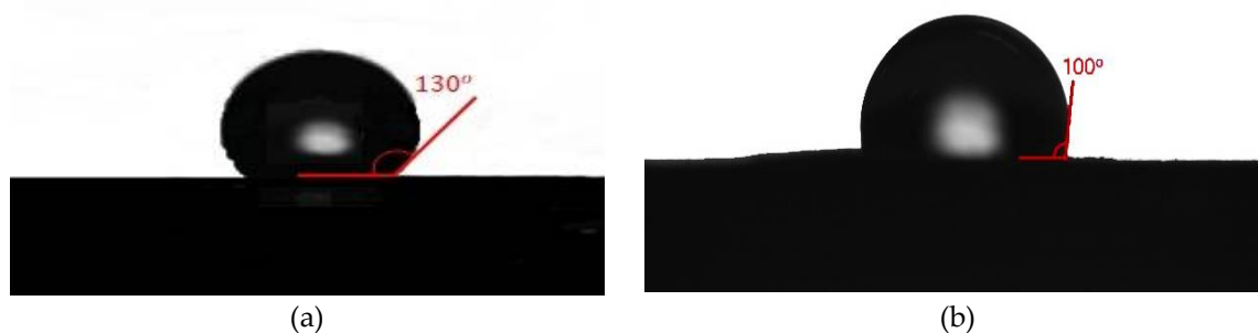
Figure 5. Contact angle: (a) water droplet on PVDF membrane surface [36]; (b) methylene blue droplet on PVDF membrane surface.
