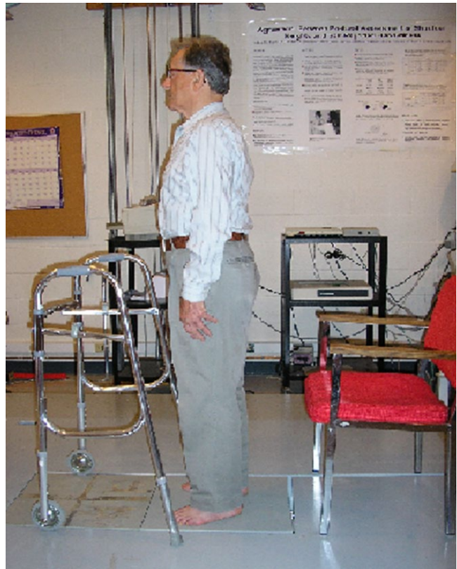
Figure 1. Participant in two-limb standing position on the force plate for balance testing.
