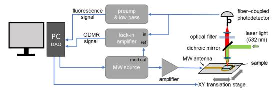
**Figure 1.** Schematic diagram of the experimental setup. A home-built confocal microscope is used for NV fluorescence detection. ND samples are placed on top of a loop-gap-type antenna and the magnetic resonance is observed for frequencies around 2.9 GHz.
