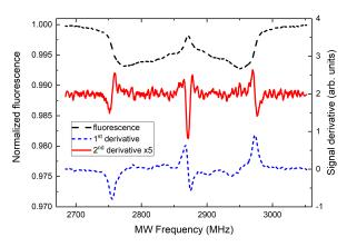
**Figure 3.** ODMR signals used for magnetometry: spectrum in 3.7 mT field from Figure 2c (dashed black) and its first (dotted blue) and second (solid red, vertically offset) derivatives. Zero-crossings of both the latter signals are independent on the fluorescence intensity and may be used for temperature and magnetic-field sensing.
