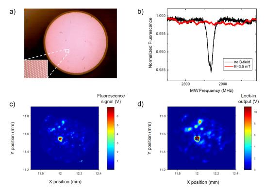
**Figure 4.** Remote sensing using IFB with a ND-coated distal facet located close to the MW antenna surface. (a) Optical microscope image of the fiber bundle. (b) ODMR spectrum measured through a single fiber of the IFB in zero and non-zero magnetic fields exhibiting single-crystal type resonances. (c,d) Fluorescence and the corresponding ODMR contrast maps acquired by scanning the proximal end of IFB.
