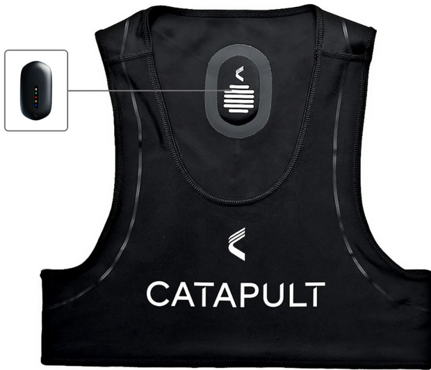
FIGURE 1. The Catapult Vector GPS monitoring system collects physical load data through embedded compact units worn in halters by each study participant during regular participation.
