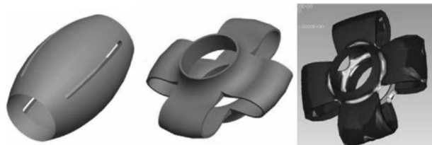
Fig. 8 Expanding four slit restraint sock: (a) restraint off; (b) restraint on, and (c) FEA of expanded sock
