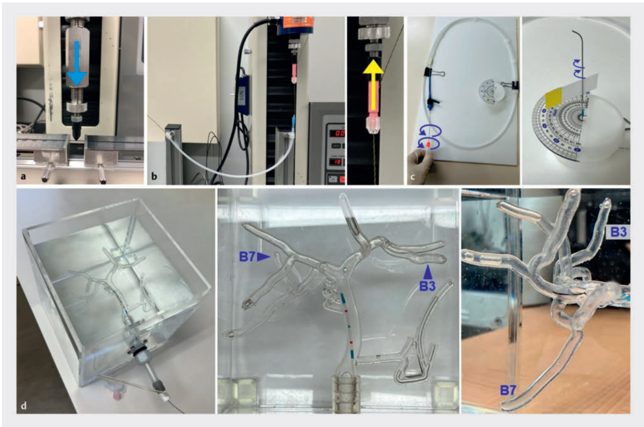
► Fig. 2 Performance tests. a The three-point bending test using the universal testing machine. The shaft stiffness (bending force) of the guidewire is measured. b Measurement of shaft lubricity of guidewire in the catheter using the universal testing machine. The maximum friction force is measured as the guidewire is pulled inside the catheter. c The torque response of the guidewire is measured. Rotation is applied from the distal side of the guidewire in the circumferential direction, and the angle of rotation required to rotate the tip 30° is measured. d The 3D-printed silicone bile duct model. Twenty endoscopists participated in the seeking test to determine the insertion success of each guidewire. The target branches are B3 and B7.
