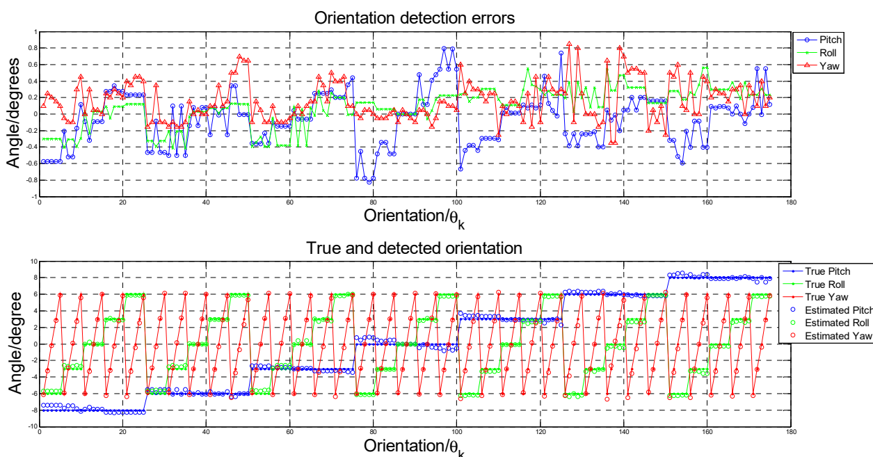
Figure 9. (Upper) Orientation detection errors for each orientation \theta_k . (Lower) the true and detected angles for each orientation \theta_k .
