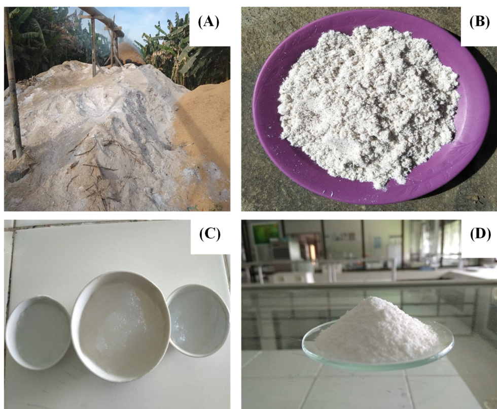
Figure 1. Rice husk ash can be processed into silica particles. (A) Bulky rice husk ash, (B) rice husk ash sample, (C) silica gel obtained from rice husk ash, (D) silica particle prepared from rice husk.
