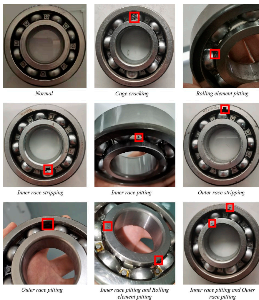
Figure 9. Schematic diagram of rolling bearings in nine health modes. The internal fault position of the rolling bearing corresponds to the marked position.
