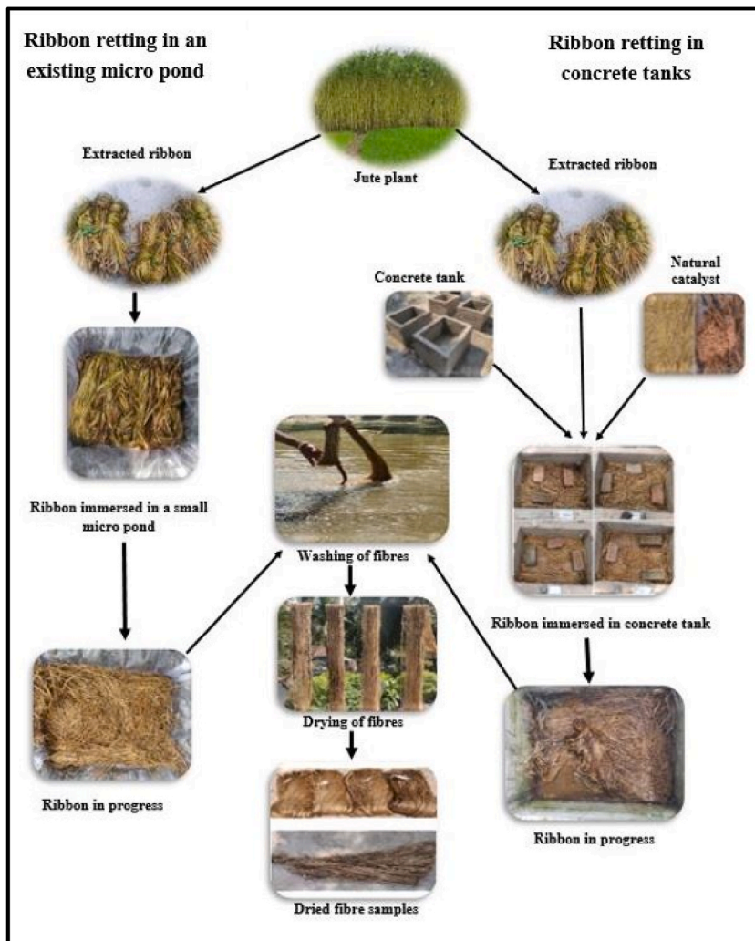
Fig. 8. Schematic diagram of ribbon retting in an existing micro pond and concrete tanks.
