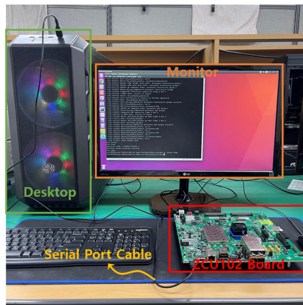
Figure 11. Photograph of the entire system consisting of the PC and ZCU102 board including the proposed accelerator.
