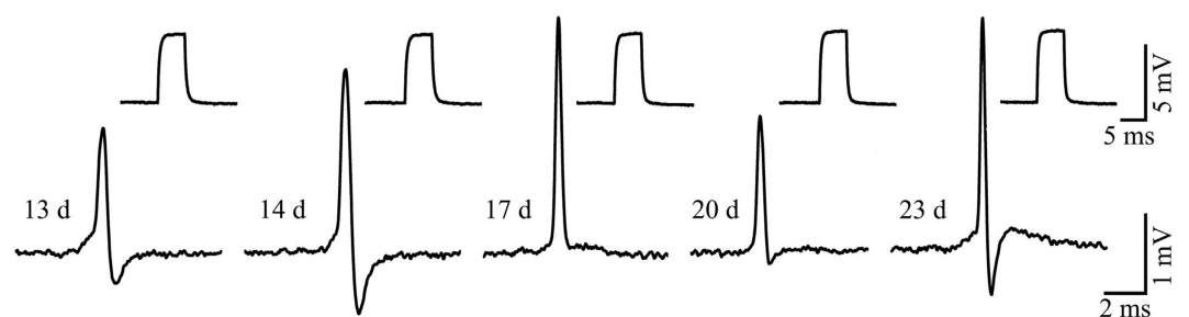
Figure 3. Changes in the shape and amplitudes of spontaneous action potentials recorded by one gM \mu E over a period of 10 days. Note that the amplitude and shape of the calibration pulses did not change, indicating that the electrode properties remained unaltered during the experiment.
