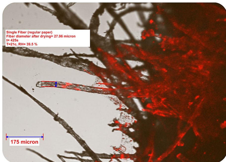
Fig. 14 Swollen of a single cellulose fiber
