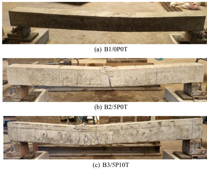
Figure 9. Crack patterns and failure modes of beams.
