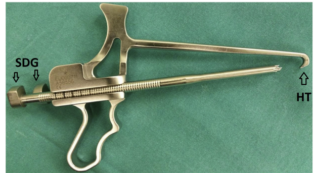
Fig 2. The glenoid guide. Glenoid guide with special bullets used to make the bony tunnels from posterior to anterior at level of glenoid rim and two 2.8-mm sleeves (specific instruments created by Smith & Nephew). (HT, hook tip; SDG, sleeved glenoid drill.)
