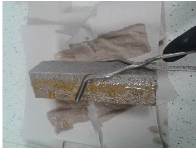
Figure 31. Gel substance on ZIII mortar exposed to 5% hydrochloric acid solution after 365 days.
